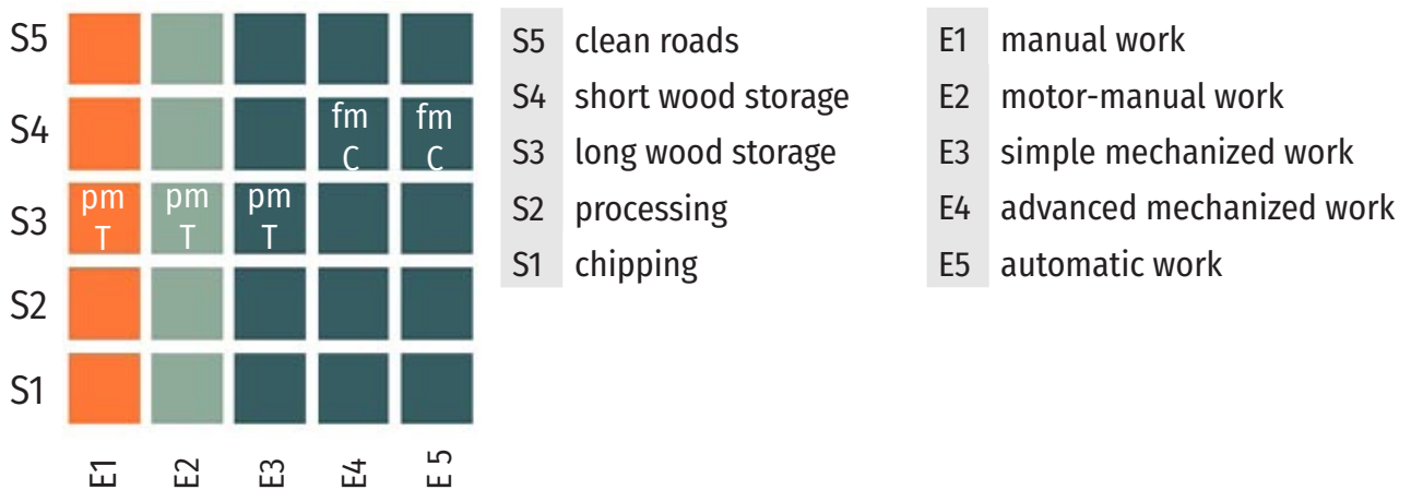
Figure 77: Example of ergonomic preference: The decision-maker prefers mechanized work (dark green) and does not accept manual work (orange)
